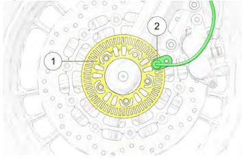
Inspect for debris adhering to the end of the wheel speed sensors (2). If contamination is observed, or if you are unable to visually inspect, slide a thin towel across the face of the sensor between the sensor and the tone ring to remove any potential debris.
