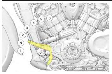
Press downward on the toe lever to shift to a lower gear. Lift upward on the toe lever to shift to a higher gear. Release the clutch lever after each gear shift.
