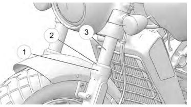
2. Clean the fork tubes to remove bugs, tar or buildup which may cause seal wear or leakage. Inspect the outer surfaces of the inner fork tubes for scratches or damage from foreign objects.
