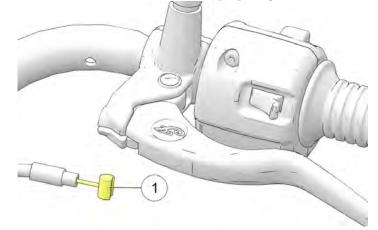
3. Reconnect the cable and adjust freeplay as needed.
