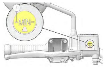
3. The fluid level should be above the minimum indicator mark in the sight glass.
