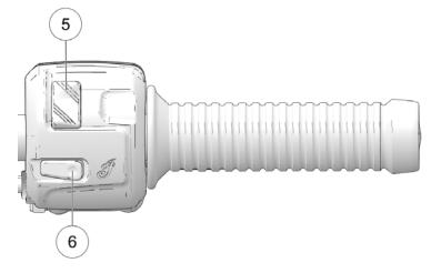
(5) Engine Stop/Run Switch(6) Engine Start Switch
