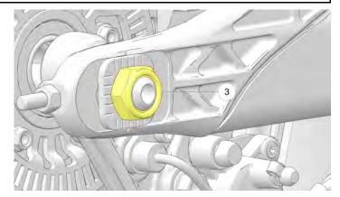
3. Turn **LEFT SIDE** adjuster nut ④ to achieve proper belt tension.
