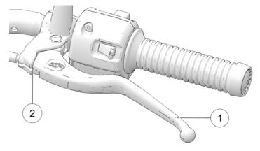
2. Freeplay (gap) is the amount of lever movement from the rest position to the point of cable resistance. Clutch lever freeplay should be 0.5-1.5 mm. Measure the gap between the clutch lever and the lever housing ②. See page 94. Adjust clutch lever freeplay if necessary.
