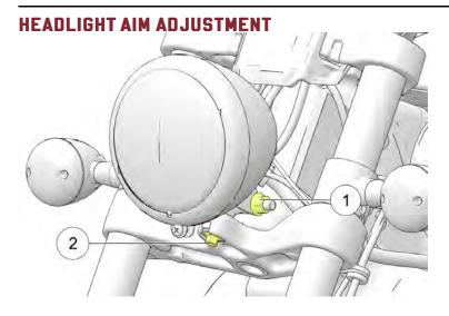
1. To adjust the headlamp vertically, loosen the housing mount fastener (1) and pivot the housing upward or downward. Tighten the fastener.
