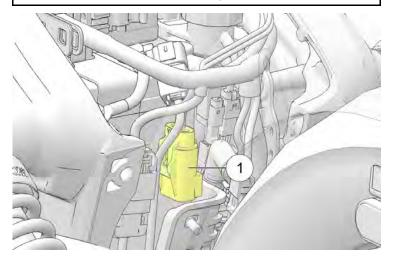
The standard fuse box is located under the seat. This fuse box houses all standard service fuses and the automatic circuit breakers. Fuse application and size are provided on a label on the fuse box cover.
