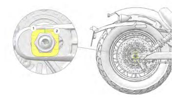
2. On right side of motorcycle, loosen the axle nut ③. Retighten to Adjustment Specification.
