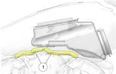
Inspect the crankcase breather (vent) hoses ① each time the fuel tank is removed to perform air filter service or other maintenance. Inspect both breather hoses along their length and at both ends. Make sure hoses are not restricted, kinked, cracked or otherwise damaged. Replace any worn or damaged hoses.
