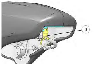
9. Gently feed fuel rail end of the fuel hose toward the center of the vehicle. Ensure the hose and connector are clear of coolant hose and all wire harnesses.
