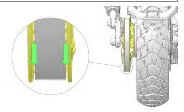
2. Rotate wheel **FORWARD** and verify sprocket teeth are still visible on both side of drive belt.
