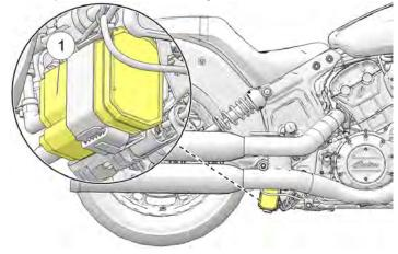
3. Inspect connections at the evaporative emissions canister to be sure they are secure.
