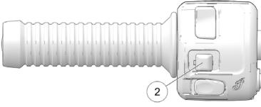
To activate the hazard switch, press on the center of the turn signal switch (2).
