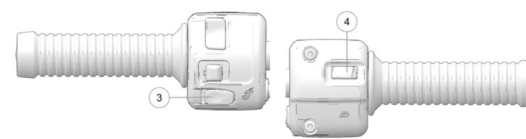
Use the Mode switch to set the display units to either standard or metric units of measurement. See the *Multi-Function Display (MFD)* section for details.
