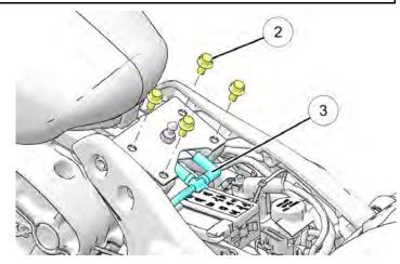
8. Connect the fuel tank vent line and the fuel cap recess drain line ③.
