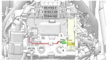
4. Disconnect the wiring harness from the upper battery tray by removing it from the two retention areas and move it off to the left side of the bike.
