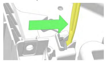
7. Install the battery hold down strap fastener 3 through the battery hold down strap 2.
