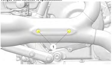
TORQUE 7.4 ft-lbs (10 Nm) Check the two muffler clamps  $\scriptsize{\textcircled{\scriptsize 1}}$  . Torque each clamp to specification.
