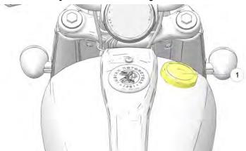
Turn the fuel cap counter-clockwise to remove it. If the fuel cap is equipped with a tether, carefully rest fuel cap on the tank so that the rubber bumper is contacting the tank. See page 80 for fueling instructions. To tighten the cap, turn it clockwise until the seal compresses onto the tank, then continue to tighten until the cap ratchets several times.
