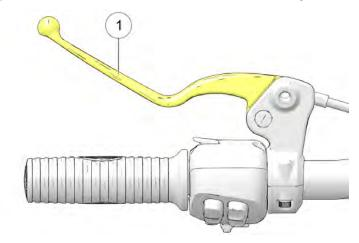
2. Freeplay (gap) is the amount of lever movement from the rest position to the point of cable resistance. Clutch lever freeplay should be 0.5-1.5 mm. Measure the gap between the clutch lever and the lever housing ②. Adjust clutch lever freeplay if necessary.
