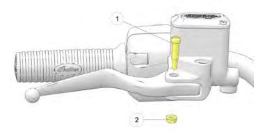
2. Install the pivot pin 1. Torque the pivot pin to specifications.
