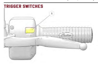
There are trigger switches located on the reverse side of both the right and left 1 switch cubes.
