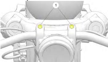
3. Rotate the handlebar into the desired position and torque the riser clamp fasteners to specification.
