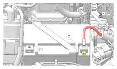
9. Remove the fastener ® securing the battery strap 9.
