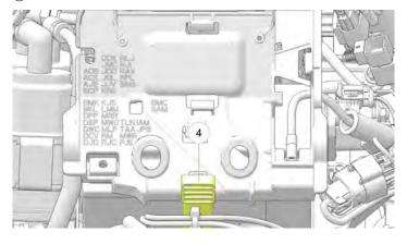
9. Install the negative (-) cable ③. Route the starter ground cable beneath the frame ground cable on the negative battery terminal.
