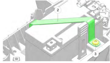
TORQUE 84 in-lbs (9.5 Nm) 8. Install the battery cover. Secure the cover with the cover strap  $\P$ .
