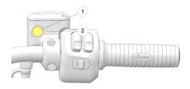
6. Reinstall the diaphragm, diaphragm plate, and screws.
