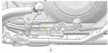
3. Turn the cable adjuster nut inward or outward until clutch lever freeplay is 0.5-1.5 mm as measured at the clutch perch.
