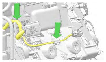
11. Install the antenna  $\mbox{\Large (6)}$  onto the upper battery tray. Connect the antenna harness  $\mbox{\Large (7)}$  to the antenna.
