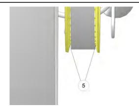
If necessary, loosen the axle bolt and LEFT SIDE adjuster until belt just moves off the right flange and begins to track down the center of the driven sprocket flange during forward wheel rotation.
