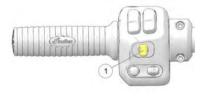
One arrow flashes when the corresponding turn signal is activated. Both arrows flash when the hazard signal is activated. If there is a problem in the signal system, the lamps will flash at twice the normal rate.
