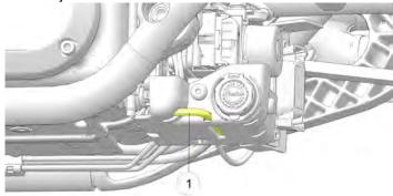
3. On models equipped with a passenger seat, remove the rear seat bracket bolt ①, washer, and nylon grommet.
