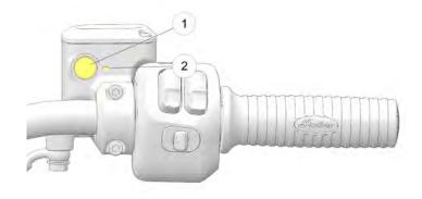
The fluid level should be above the minimum indicator mark (2) in the sight glass.
