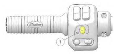
To activate the hazard switch, press on the center of the turn signal switch  $\widehat{\textbf{1}}$ .
