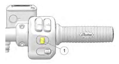
Cruise control can be activated and adjusted from the right control using the Cruise Control Switch ①.
